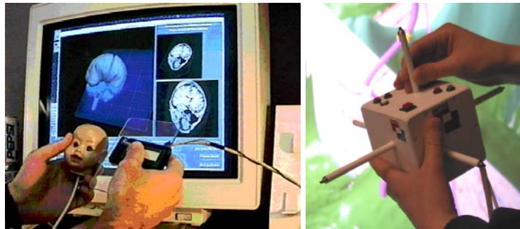
Figure 8: Tangible Interface for Navigation: Passive Props [28] and Cubic Mouse [22].
