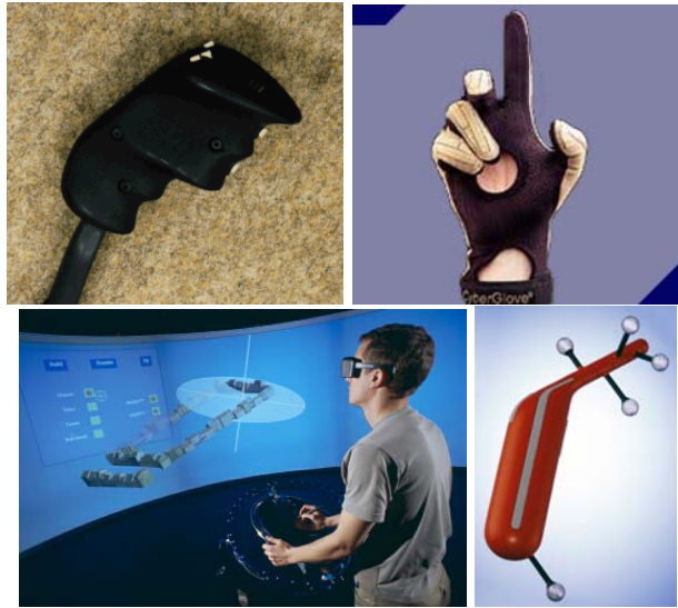
Figure 6: 3D Devices: traditional (top, 3d mouse cyberglove) and new devices (bottom, CAT [27] and Cyberstylo©[21])
