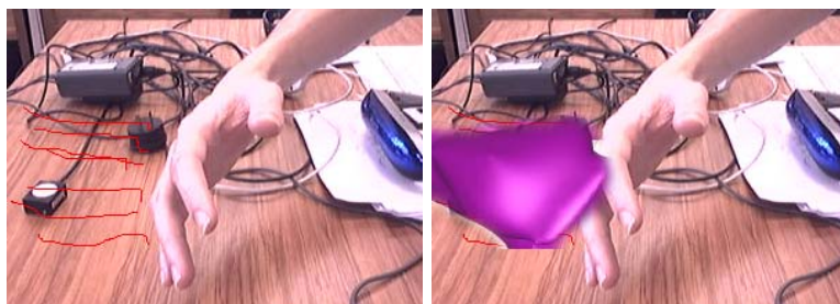
Figure 17: 3D sketching: the user can not only define 2D shapes but also create 3D curve shapes based on a meshing extrapolation between the 3D flow field.
