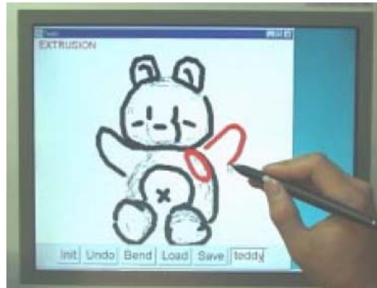
Figure 12: 2D Based-Approach: Teddy [32] software uses a simple inference rule to simply generate curved meshes
