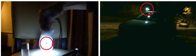
Figure 3: Our tracking algorithm automatically finds the center of the light sources with different sizes, occlusions and reflections.
